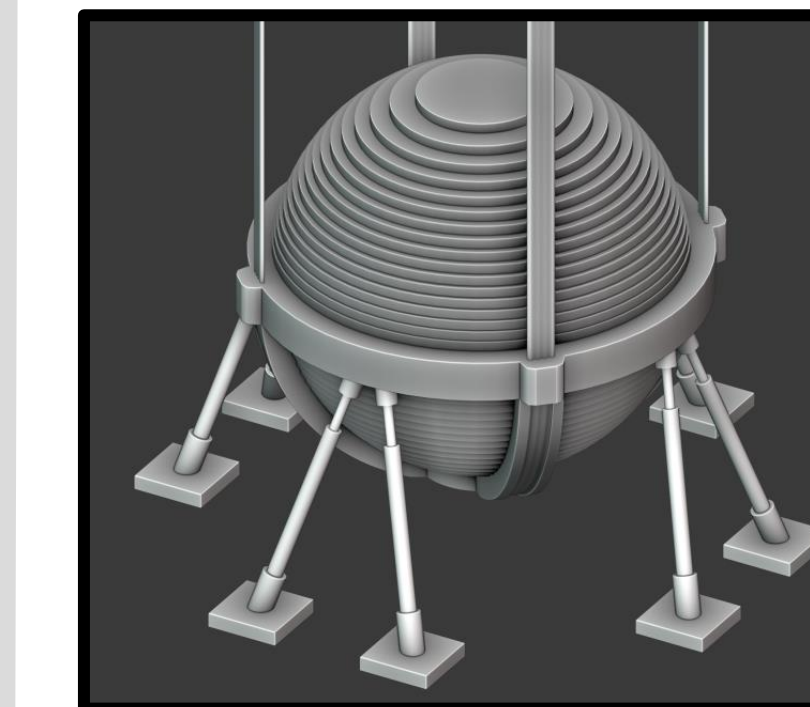
Fig. 5. Model of a TMD
